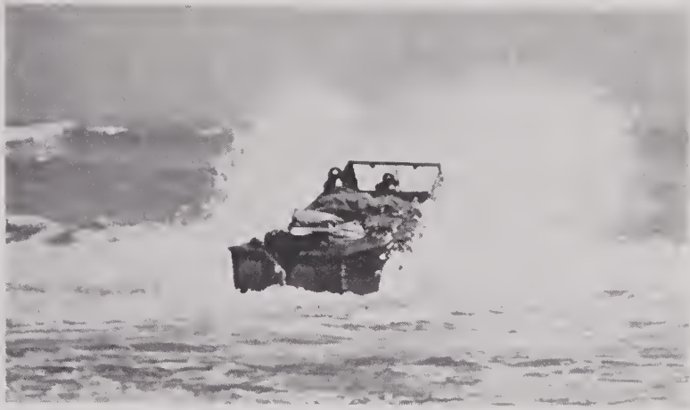
FIGURE 12. Pilot model 1/4-ton, 4x4 amphibious jeep entering moderate surf.
